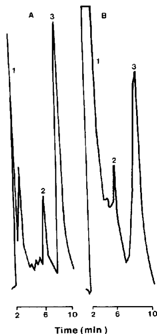
Fig. 5. Chromatograms of serum and urine from a normal subject (same as in Fig. 4) 24 h after ingestion of Oltipraz, 2 mg/kg body weight. (A) Serum (11 ng/ml); (B) urine (10 ng/ml). Peaks: 1 = solvent front; 2 = Oltipraz; 3 = internal standard. Attenuation = 0.002.
